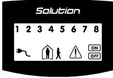
The codepad incorporates numerous indicators. There are ZONE indicators which are used to show the condition of each zone and four others for general status. The following is a list of situations and the relevant indications that will be seen.
